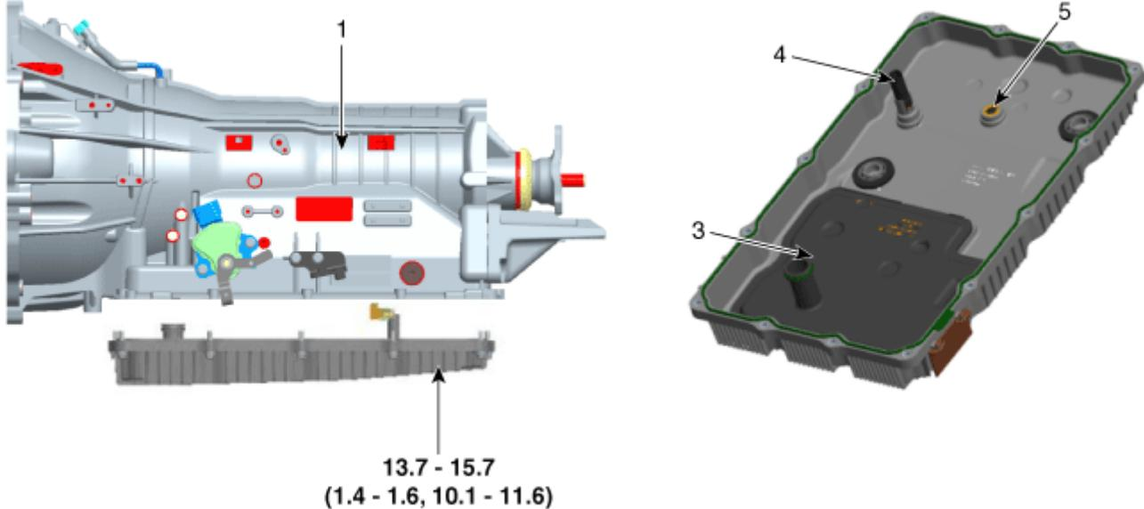
**Tightening torque : N·m (kgf·m, lb·ft)**
